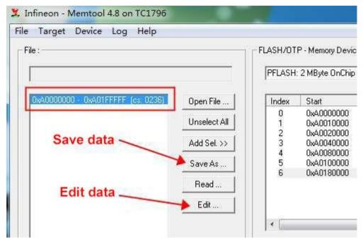
5. Chip programming: It is also necessary to ensure the correctness of the programmer driver, hardware connection, and target board environment. You must first execute Connect to ensure that the device is successfully connected to the target chip.
