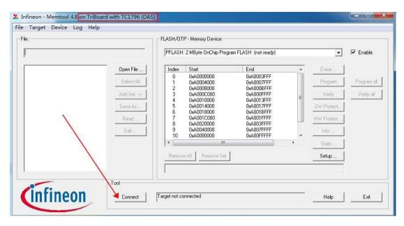
Before starting chip read/write operations, you must first execute Connect to ensure that the device is successfully connected to the target chip: The Connect button on the software interface will change as shown in the figure below, indicating that the connection to the target is successful and you can perform read, erase, write, and other operations.
