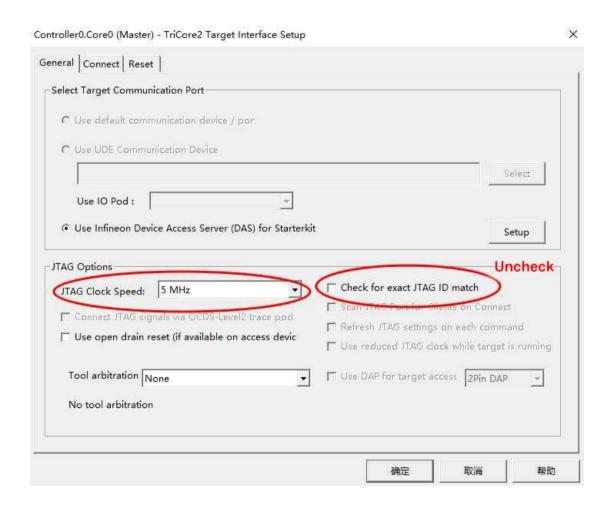
4. If you cannot connect to the target chip, you can first use the background scanning software to confirm whether the power supply and interface connections are correct. Locate and run C:\Program Files\DAS64\clients\das\_device\_scanner.exe, →Start DAS Server →Install Servers → Start. Return to the initial interface and click Start Client. If the chip category is identified as TriCore-Family, it indicates that the power supply and interface connections are correct. Otherwise, further
