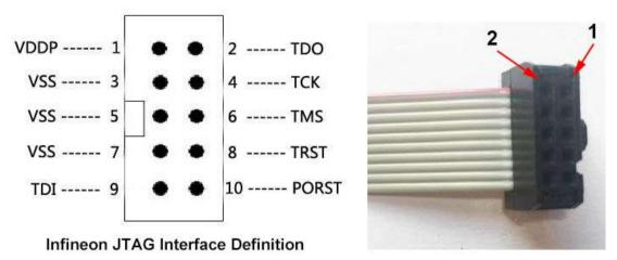
VDDP: Connect to the target chip's operating power supply 3.3V/5V. The programmer board J2 does not output
